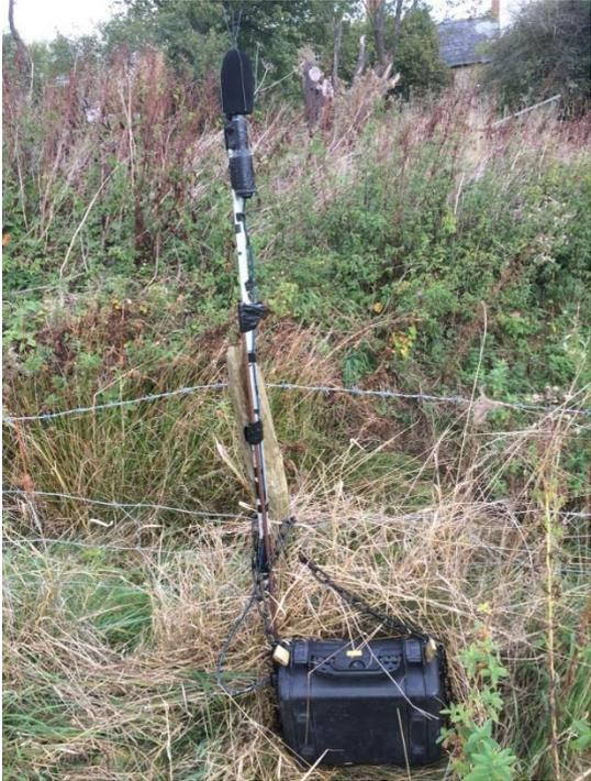
Clarke Saunders Acoustics have been appointed by Tidal Lagoon Power to record background noise levels around the proposed lagoon areas. They have installed apparatus similar to that shown in this picture on the reserve
